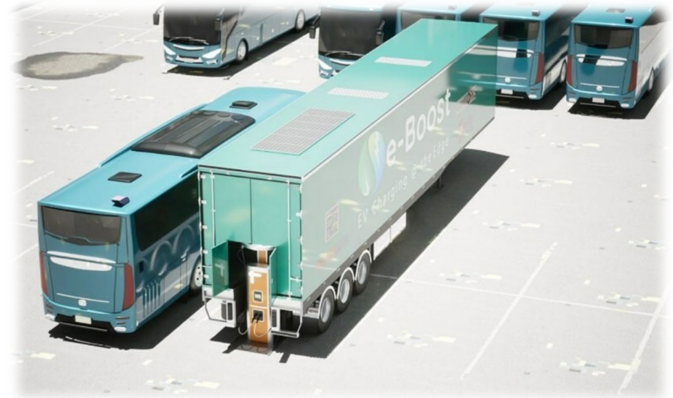
180KW off grid DC Fast Charger and genset supporting transit fleet ops
