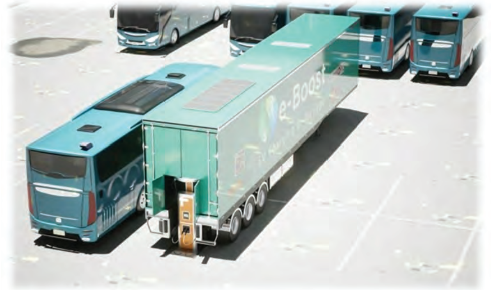
180KW off grid DC Fast Charger and genset supporting transit fleet ops
