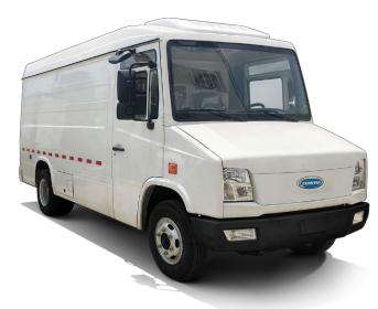
The LS 400 is an all electric Class 4 truck designed for urban delivery and logistics. It features two 40 kWh battery packs offering a range of 124 miles.
